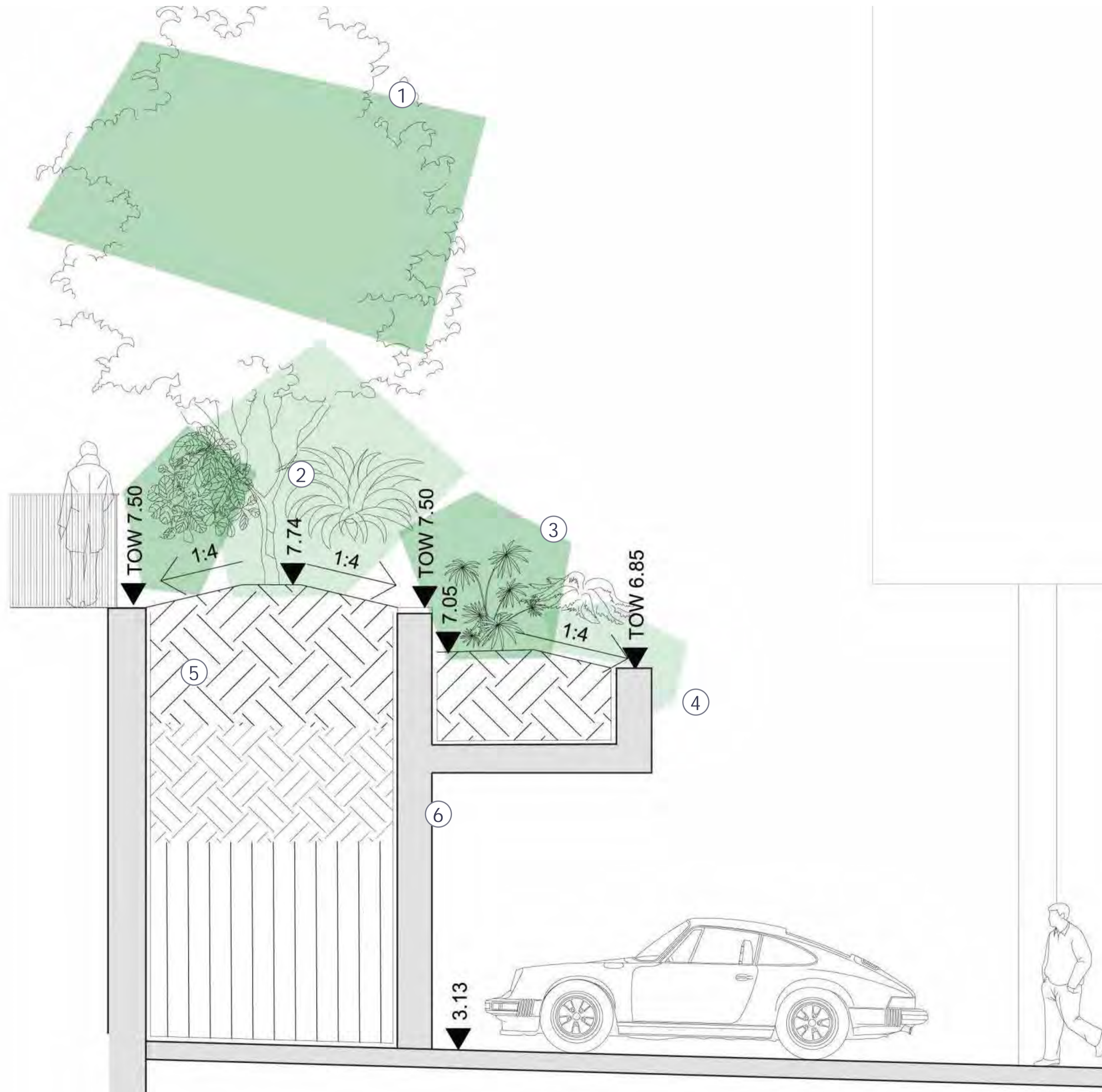
SECTION A-A (Refer to sheet DA-1846-03) Scale 1:50 @ A3
